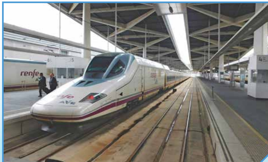
A Talgo 350 stands at Valencia on April 1, having travelled from Madrid. The trains are capable of 330kph (205mph) and entered traffic in 2005. RICHARD CLINNICK.
