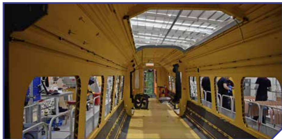
Above: Inside a newly arrived Class 196 bodysell. These are shipped from CAF's Beasain factory in this condition, with the Newport facility then fitting them out. RICHARD CLINNICK.
