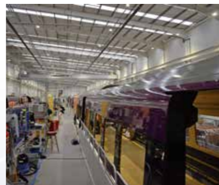
Above right: Driving vehicles from the final Northern Class 195/1 diesel multiple units await the fitting of their Rolls-Royce MTU engines (seen on pallets to the left of the vehicles) on January 30. This is one of three production lines at Newport, and will shortly be home to Transport for Wales Class 197s undergoing the same process. RICHARD CLINNICK.
