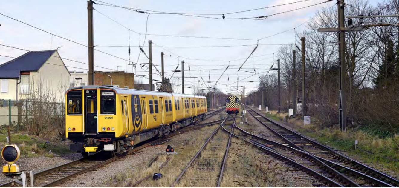
Network Rail 313121 passes Bowes Park reversing siding on February 15, with a test train from Willesden TMD to Watton-at-Stone. The train is used to test in-cab signalling and ETCS on the Hertford Loop, from its base at the Digital Railway-owned ETCS National Integration Facility at Hitchin. ANTONY GUPPY.
