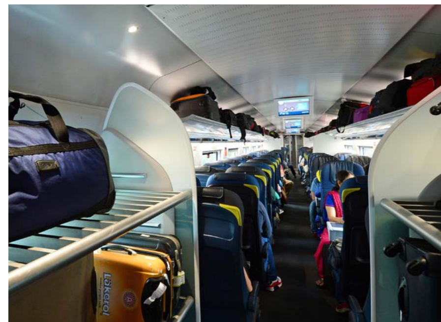
The e320s are built to European-UIC gauge so there is more luggage space. PAUL BIGLAND.
