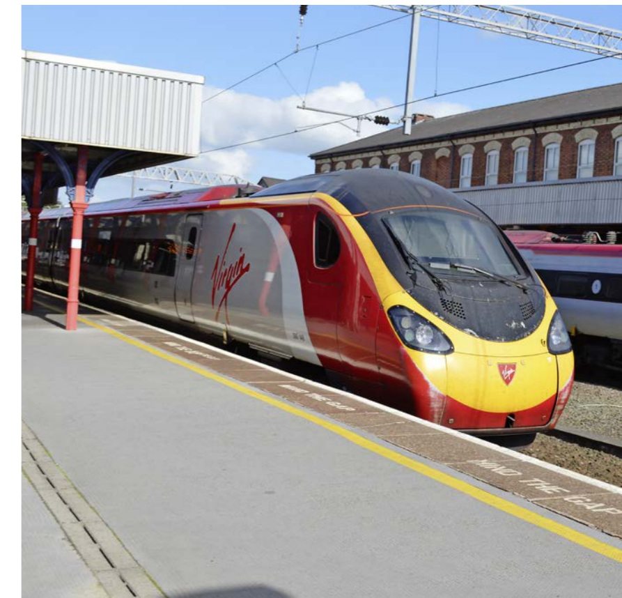
Virgin Trains 390148 forms the rear of the 1216 Stockport-Manchester Piccadilly nine-car Pendolino service on October 6. These trains are capable of running at 140mph, but are limited to 125mph by Network Rail's maximum permitted line speeds. PAUL STEPHEN.
